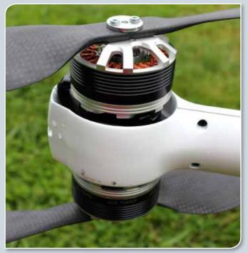
The coaxial propulsion arrangement on the SkyJibX4.
