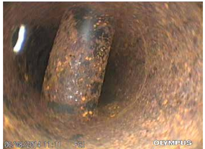
Internal corrosion on a Cessna control yoke.
