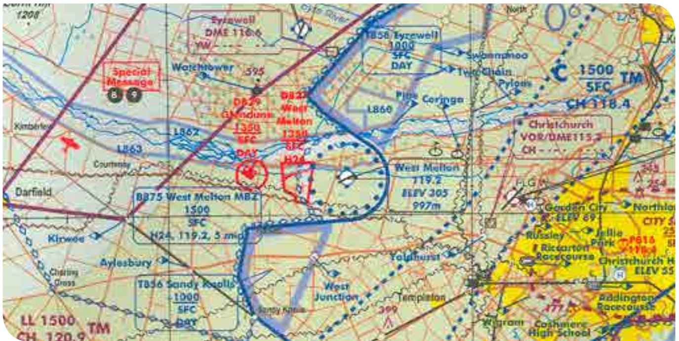
This section of VNC C13 shows the West Melton MBZ and the two transit lanes either side. There is a tendency for pilots to fly through the circuit at West Melton - see the article for advice.
