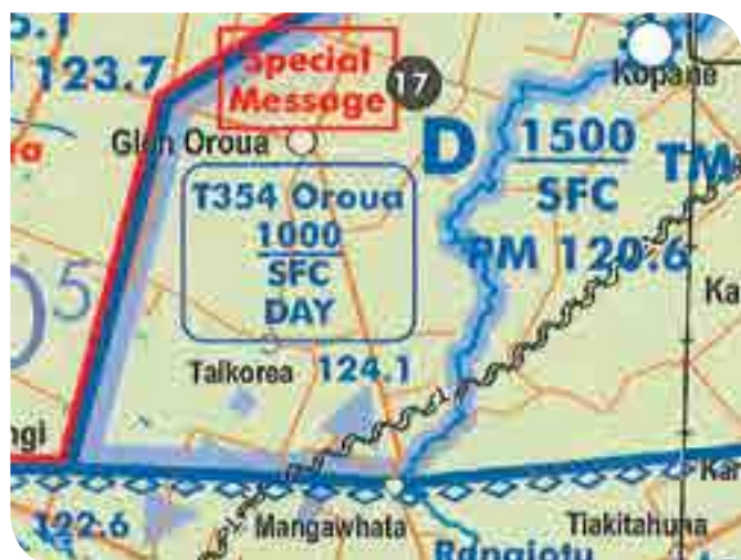
This example from VNC C2 shows the recommended T354 frequency 124.1 MHz (this is the Feilding aerodrome and CFZ frequency). Note the change to 122.6 MHz in the Manawatu CFZ to the south of T354.
