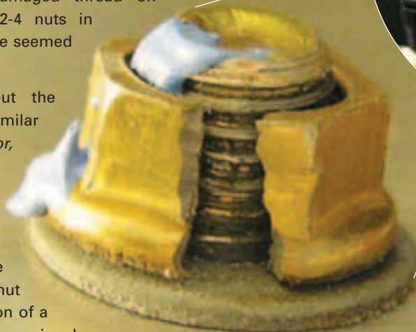
The broken MS21042-4 nut that Brian Anderson found on his brand new Jabiru engine.
