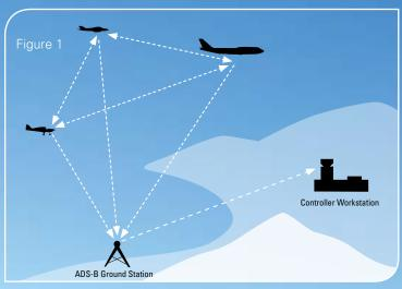
ADS-B data Broadcast at 0.5 second intervals. Sends: Position, Altitude, Identity, Velocity Vector, and Integrity Data.
