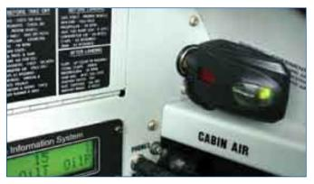
An example of a portable electronic CO detector fitted to an amateur-built aeroplane. Photo courtesy of Bob Jelley.
