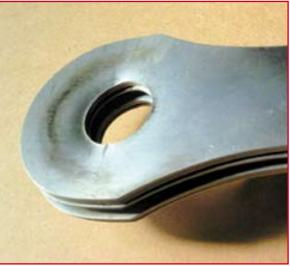
Damage at the TT strap retention pin hole.
