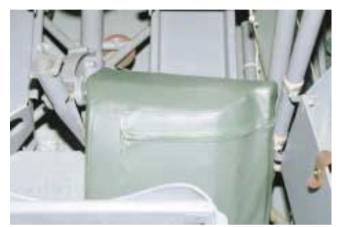
The seat cushion jammed between the fuselage and the control column stub. The rear control column is removed for solo flight. Note the angle at which the ailerons were jammed.
