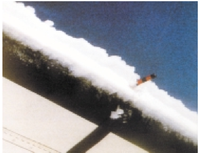
Rime ice on the leading edge of an ATR wing. It is typically very brittle and frost-like in its appearance.
