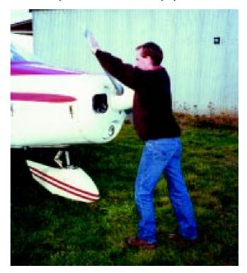
With a Gipsy engine such as on a Tiger Moth (rotating clockwise when viewed from the front) weight is transferred from the right to left foot and the prop-swinger walks away to the left (as pictured below).
