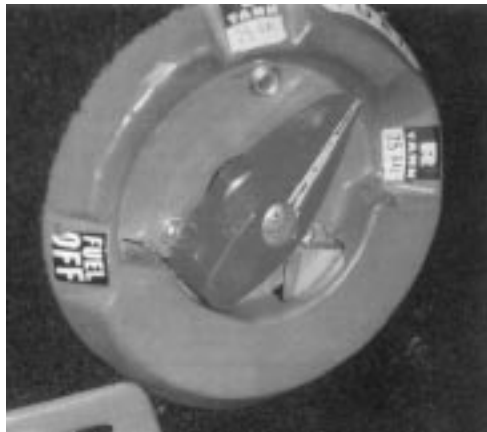
This fuel selector belongs to a British PA28-140 that experienced in-flight fuel selection problems. The selection lever could not be fully rotated to the righthand tank position due to a loose trim screw jamming its tail-end. Fortunately, there was sufficient fuel in the lefthand tank to complete the flight safely. Aircraft fuel selection units certainly do warrant an inspection from time-to-time to check their function and condition.
