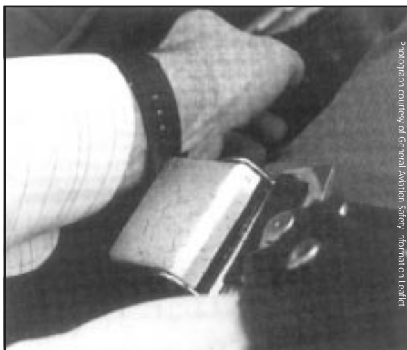
This photograph illustrates how a watchstrap, jersey or coat sleeve can unknowingly become caught under the seat belt locking mechanism and release it.
