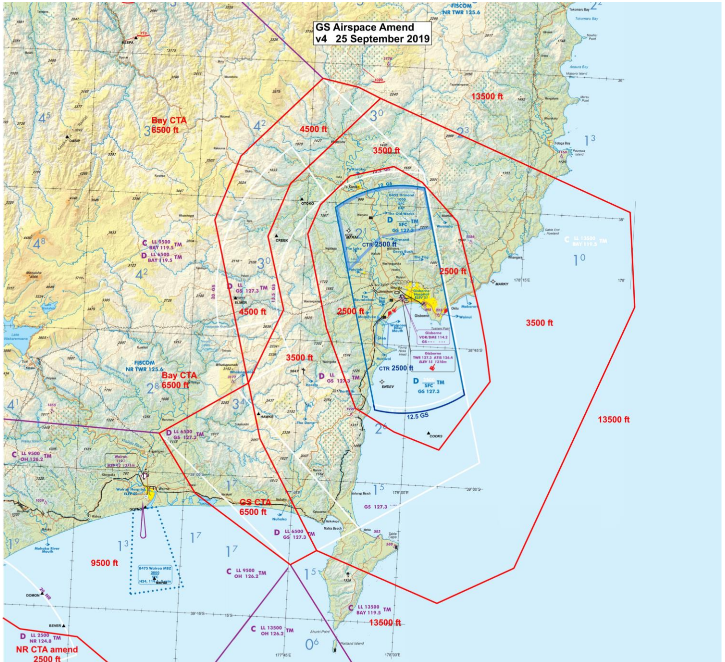
Diagram 1 DRAFT amended GS CTR and CTA version 4 Note minimal change to the GS CTR boundaries except that the upper limit is lowered to 2500 ft. White lines are the existing airspace boundaries to be deleted
