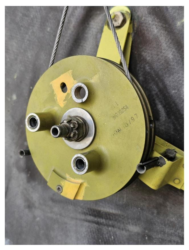
Thruster Control Output Drum Assembly P/N 500N7221-1
